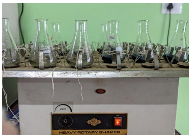
Figure 14. Shaking for 40 min in a mechanical shaker
