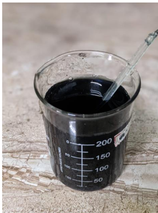
Figure 12. Beaker containing Eriochrome Black T and charcoal
