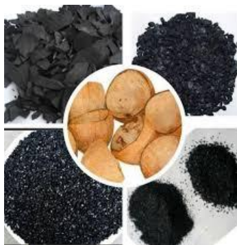
Figure 1. Schematic representation of charcoal from coconut shell
