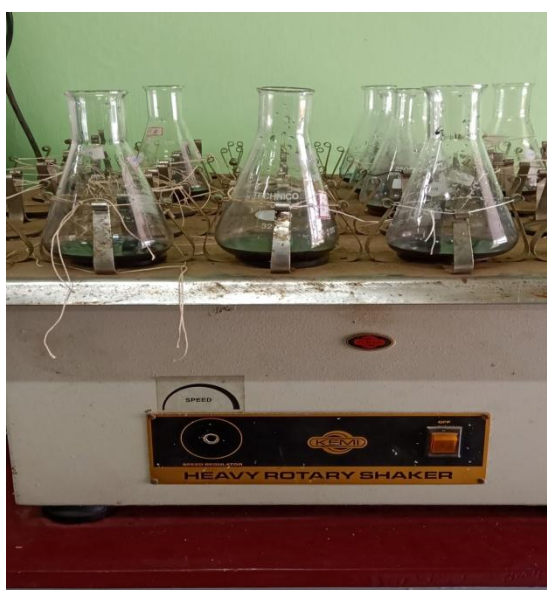
Figure 10. Batch adsorption process of Eriochrome Black T
