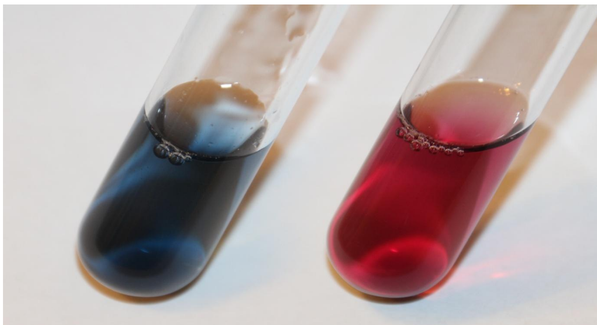
Figure 6. EBT is blue in a buffered solution at pH 10. It turns red when \text{Ca}^{2+} ions are added.
