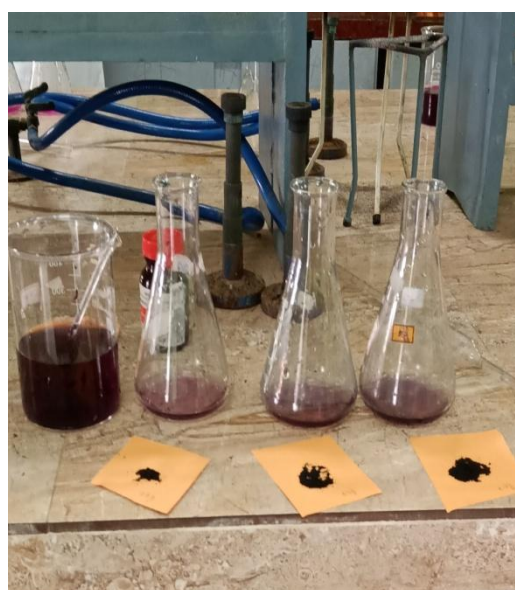
Figure 10. Batch adsorption process of Eriochrome Black T
